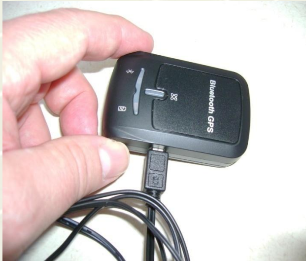
Traffic Management System contains third-Party low-end WAAS GPS Receiver
