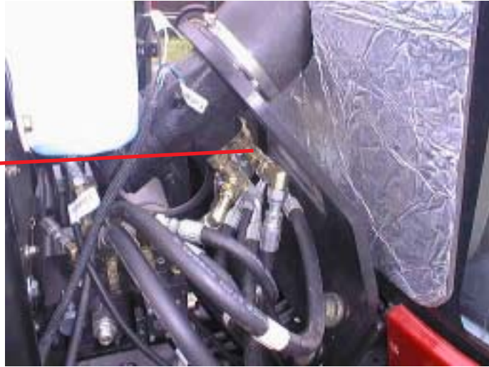
Left steer hose connection to orbital tee fitting
