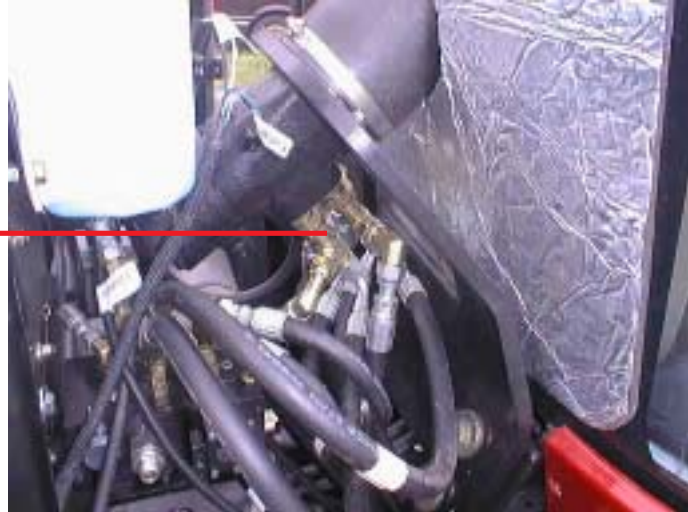
Right steer hose connection to orbital tee fitting
