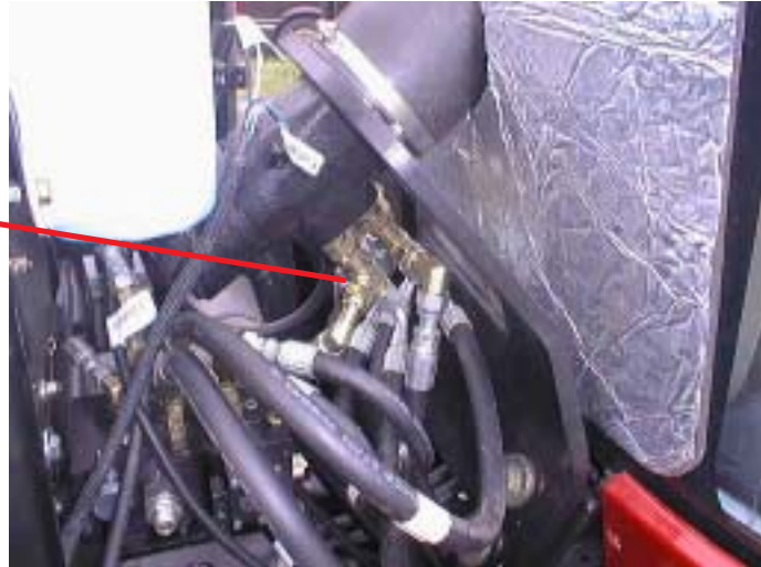
Pressure hose connection to orbital tee fitting
