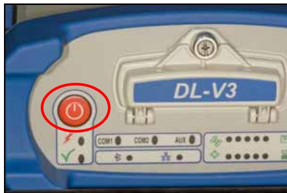
FIGURE 3. Slingshot Base Station Modem Power Button
